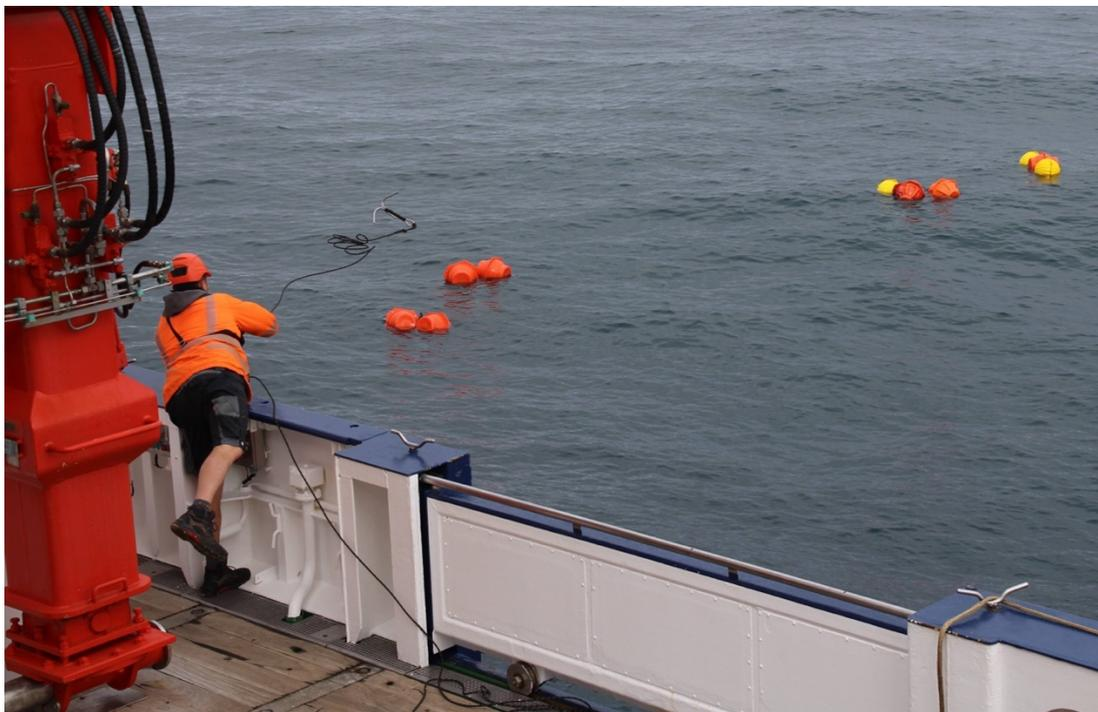
*Fig. 4.4: A grapnel is used for the recovery of a mooring. Photo: Dragonfly Leathrum-Simons*
