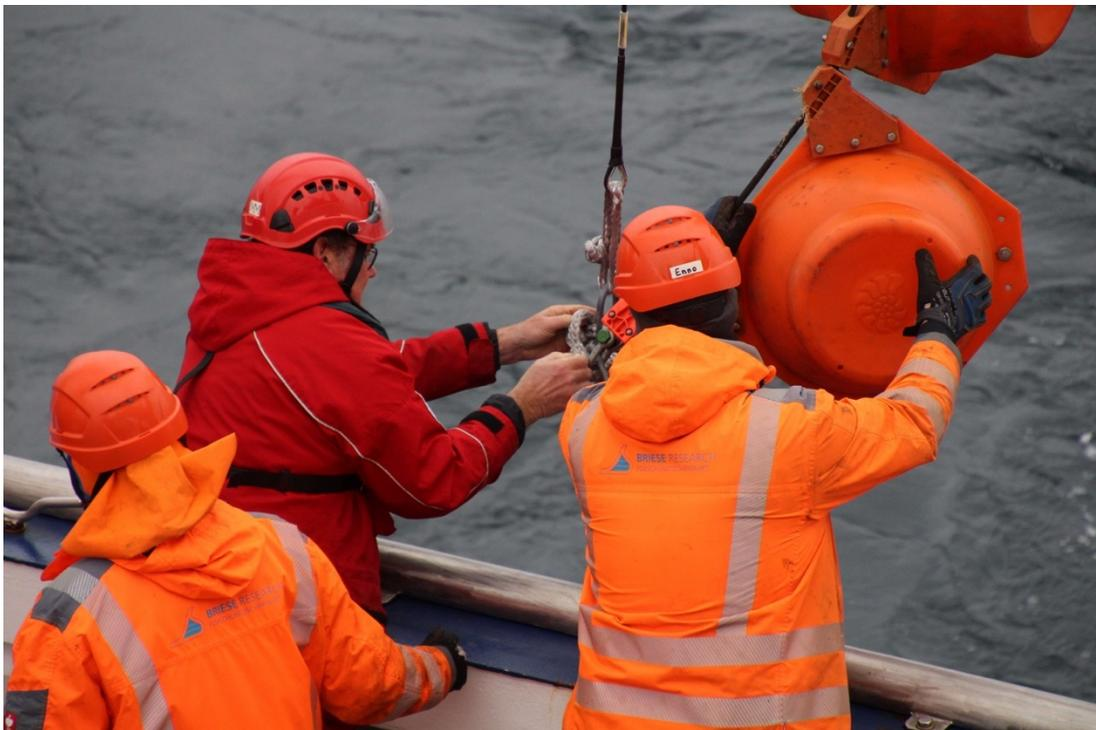
*Fig. 4.6: Deployment of a mooring in the West Spitsbergen Current over the stern of Merian (Photo: Dragonfly Leathrum-Simons).*
