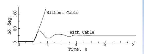
The cable links is preventing post fault voltage collapse and improves transient stability for the whole network!
